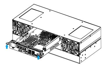
2. Secure the controller by fastening the two retention screws (1) under the ejection levers (2).
