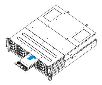
Once fully inserted, close the tray and use a small-size flat blade screwdriver to turn the bezel lock from unlock to the lock position.
