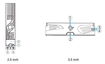
The drive tray is designed to accommodate separately purchased SAS, NL-SAS or SATA interface hard disk drives. There is a rotary bezel lock (1) that secures the drive tray in chassis, while a release button (2) can be used when retrieving disk drives from the chassis. To the right of the bezel plate, there is a drive busy LED (3) and a power status LED (4).
