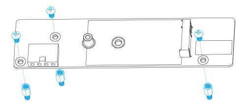
Insert the SSD at a 45 degree angle, make sure the notch meets (indicated by the blue circle). Gently lower the other end of the SSD and secure it with a screw.
