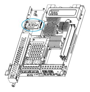
3. Flick the clips holding down the FBM in the direction of the arrow to release it and remove it while holding it on a 45 degree angle.
