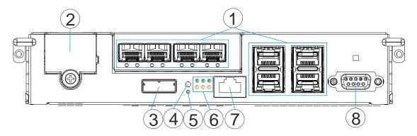
The controller on the dual controller models also features a Cache Backup Module (CBM), consisting of a Battery Backup Unit (BBU) and Flash Backup Module (FBM). The CBM and its components may be optional items for some systems.
