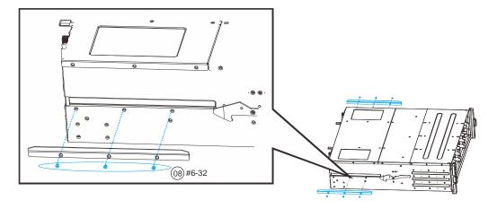
4. With the assistance of another person, lift and insert the enclosure onto the slide rail.
