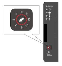
Make sure a unique ID is configured on each JBOD so that the SAS WWN addresses of disk drives can be properly assigned. RAID system firmware automatically manages these addresses.
