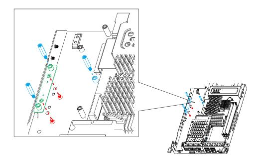
Lower the PCB board onto the controller while matching the holes to the copper stands and secure it using the supplied truss head screws.
