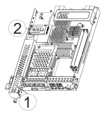
For dual controller systems, the Cache Backup Module may be a standard feature pre-installed into the controller and an optional accessory for single controller models. The Battery Backup Unit (BBU) can be serviced by the user but the Flash Backup Module (FBM) is not serviceable by the user.
