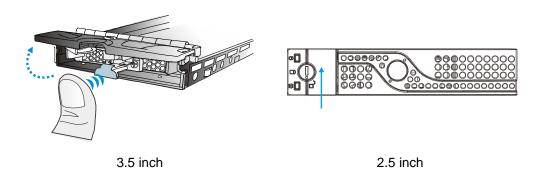
Place the hard drive into the drive tray, making sure that the interface connector is facing the open side of the drive tray and its label side facing up.
