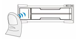
Place the hard drive into the drive tray, making sure that the interface connector is facing the open side of the drive tray and its label side facing up.
