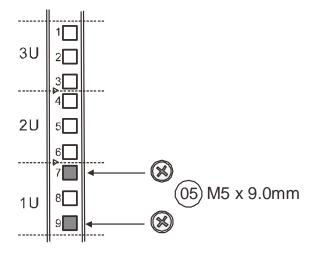
2. Adjust the length by loosening the four screws on the slide rail. Secure the slide rails to front and rear posts using truss head screws. Tighten the four screws on the slide to fix the length.
