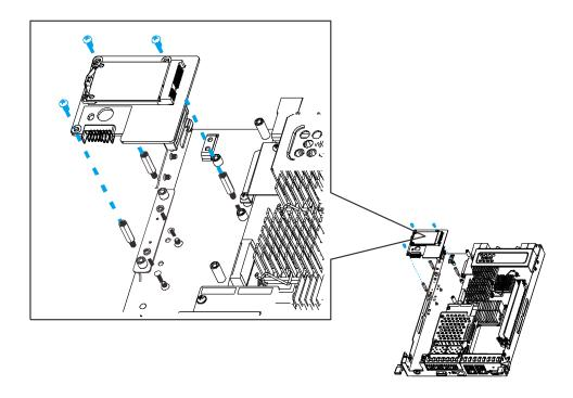
Hold the SSD on a 45 degree angle, match the notch (indicated by the circle), insert the SSD gold fingers into the slot, lower the other end of the SSD until the edges are clipped-on.
