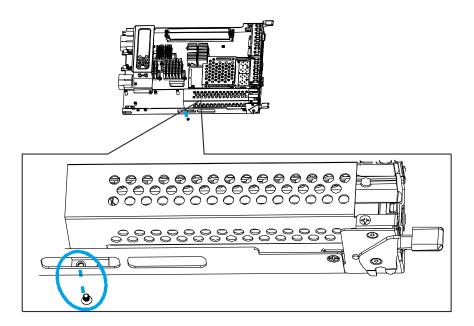
4. Gently insert the battery backup unit into the cage and secure it using the thumb screw.
