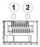
Each controller module houses fibre channel host ports. Each of these ports has two LEDs for displaying the operating status.
