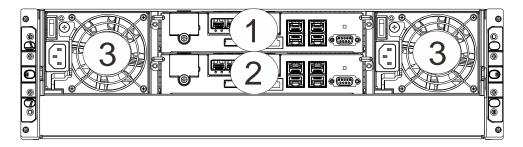
• Controllers (1) / (2): Each RAID controller module contains a main circuit board and a pre-installed DIMM module. For single controllers, a dummy cage will be placed at the controller (2) position. The host port configurations will vary. For details, see Rear Panel Components.
