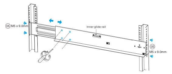
3. Attach the inner glides to BOTH sides of the enclosure using flathead screws #6-32 (8)
