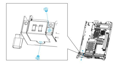
2. Hold the battery cage at a 45 degree angle, make sure the cage sits and meets the screw holes. Secure using the supplied flathead screws.
