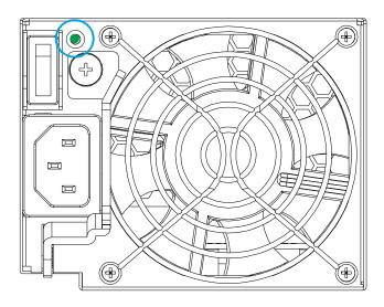
**PSU & Cooling Module Status LED**
