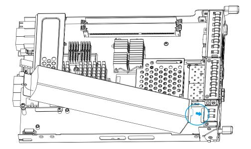
2. Secure the Super Capacitor with a supplied screw at the end (indicated by the blue circle).
