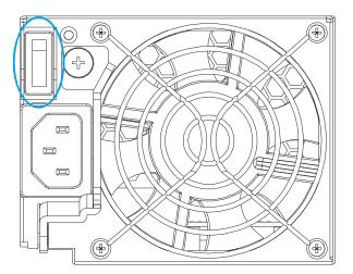
2. Loosen the retention screw that secures the extraction handle to the chassis.
