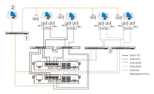
When connected to both FC host and iSCSI host, the connections will work in their respective speeds. It maximizes the number of connections while keeping the optimum performance gained by the high speed FC link and FC switch (FC).
