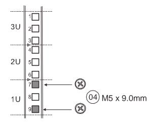
2. Install the fixed rack ear mount to the rear posts and secure them using truss head screws (4)
