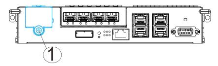
2. Using the thumb screw as an anchor, gently pull out the BBU (2).
