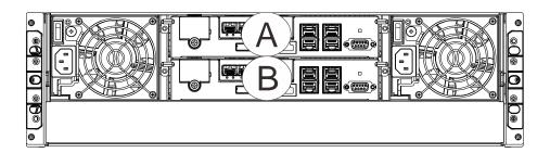
The top controller (Controller A) is the primary controller. The bottom controller (Controller B) is the secondary (= redundant) controller which is idle during normal operation and takes over the management role when Controller A cannot function properly due to hardware error, controller module removal, etc.
