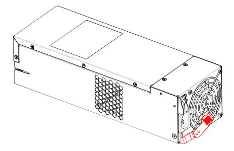
4. Insert the replacement module. Make sure the extraction handle is pointing outwards. Push the replacement PSU into the chassis, and when you feel the contact resistance, push the extraction handle towards the PSU module and it should engage the back-end connectors.
