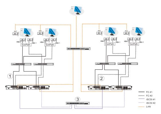
The above diagram demonstrates how to utilize the iSCSI host ports for remote data replication.
