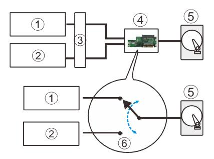
**MUX Kit Port Selector Mechanism**
